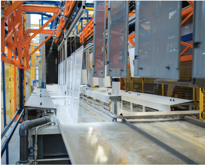
After degreasing and cleaning the sheet metal, the parts are immersed in a large vat where electrophoresis takes place.
