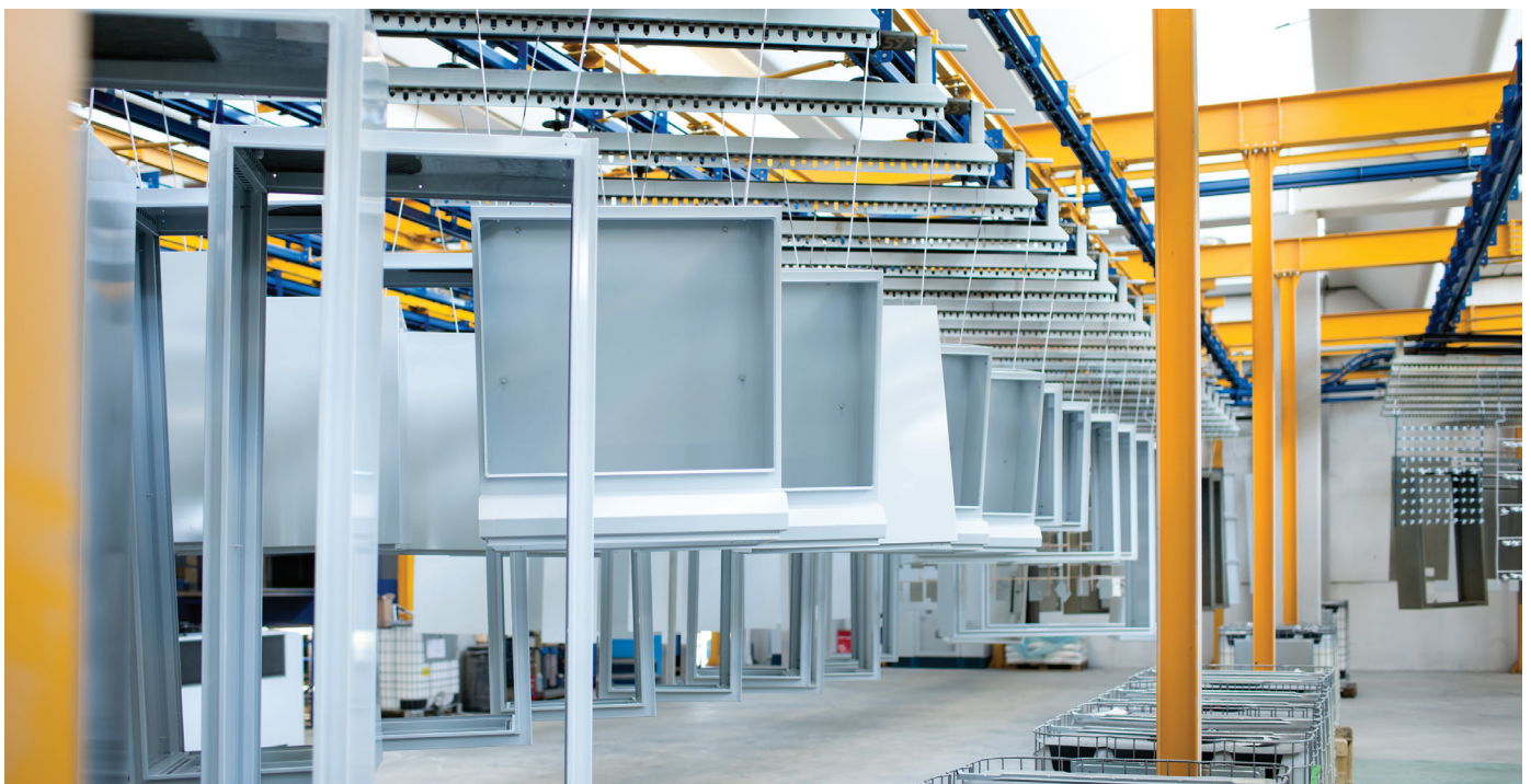
After the E DUP coating, the finished parts remain in wait of a buffer before moving on to the assembly department.
