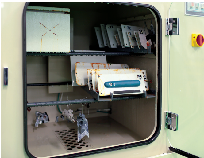
At the ETA Next's Research Centre, a chamber for saline mist is installed to test the effectiveness of the E DUP coating.
