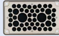
F3A-D Cellular rubber pass-through flange, 40 cables of Ø 10-13 mm, 4 cables of Ø 17-21 mm, 2 cables of Ø 27-30 mm
