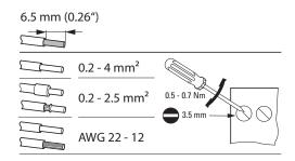
Figure 12: Screw length stripping length
