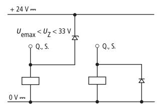
Figure 22: Inductive load with suppressor circuit
