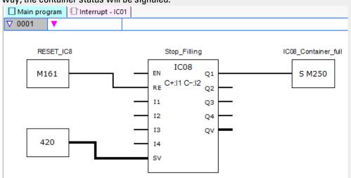
Figure 211: easySoft 7 Main program, two counter inputs
