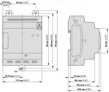
Figure 295: Dimensions in mm (Inch) base devices
