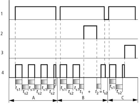
Figure 125: Signal diagram timing relay, single pulse 1
