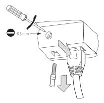
Figure 34: Removing the Ethernet cable
