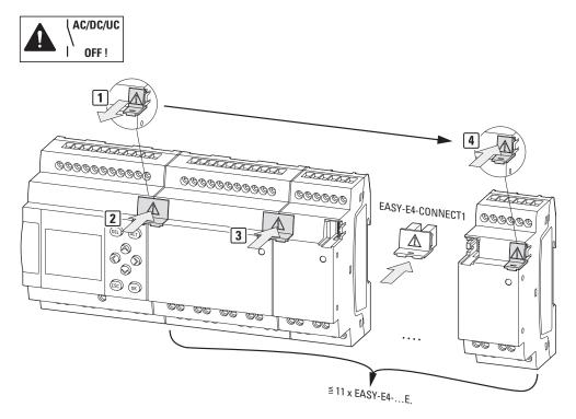
Figure 6: Assembling a base device with expansions
