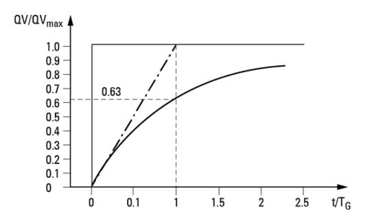
Figure 164: Response of the FT function block
