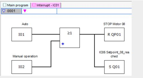
Figure 214: easySoft 7 Interrupt program Incremental counter
