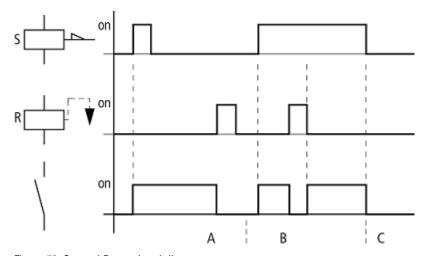
Figure 76: Set and Reset signal diagram
