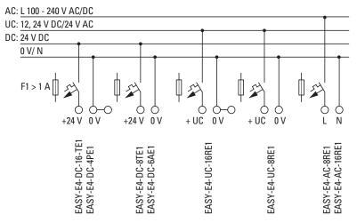
Figure 14: Connecting the power supply for expansions
