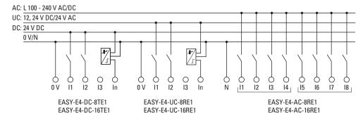
Figure 16: Connecting the digital inputs on expansions
