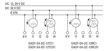
Figure 17: Connect digital counter inputs
