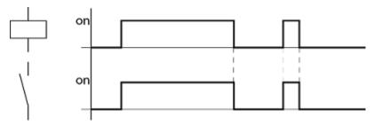
Figure 74: Contactor function signal diagram
