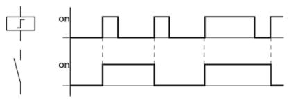
Figure 75: Impulse relay signal diagram
