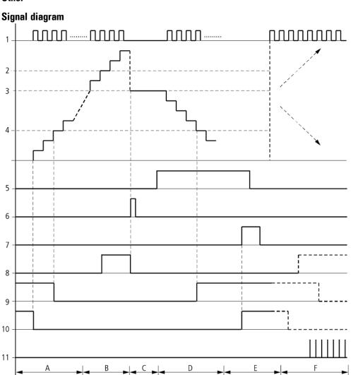
Figure 149: Signal diagram High-speed incremental value counter
