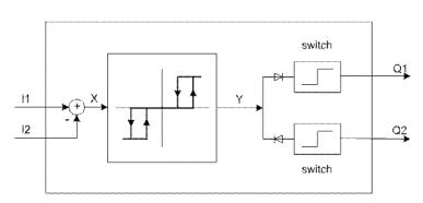
Figure 172: Three-step controller schematic diagram
