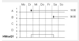
Figure 103: Signal diagram
