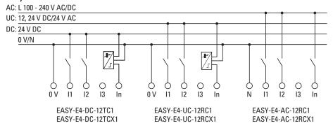
Figure 15: Connecting the digital inputs on base devices
