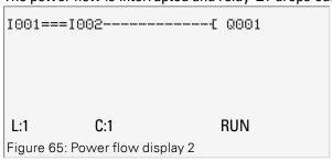
Power flow display: Input I 001 is closed, input I 002 is open, relay Q1 has dropped out
