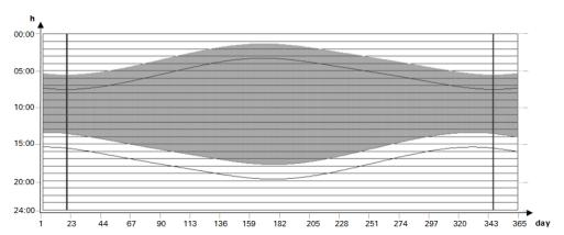
Figure 141: Offset; O1=-2; O2=-2; Q1=1 will switch on 2 hours before sunrise and off 2 hours before sunset
