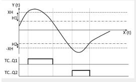
Figure 174: Signal diagram for three-step controller
