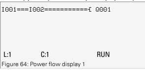
Power flow display: Inputs 1001 and 1002 are closed, relay Q1 has picked up
