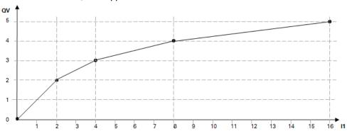
Figure 160: Example of a characteristic curve for the PM function block
