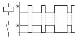
Figure 78: Inverse contactor function signal diagram
