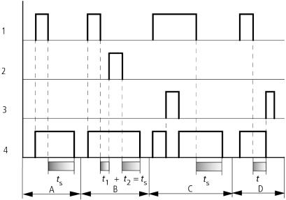
Figure 120: Signal diagram of timing relay, off-delayed
