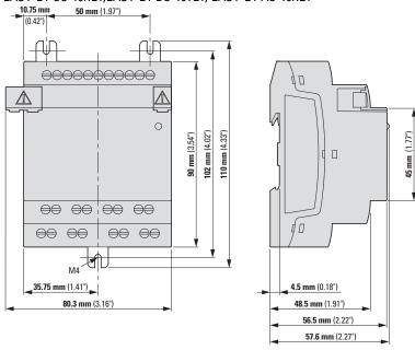
Figure 296: Dimensions in mm (Inch) extensions 4SU
