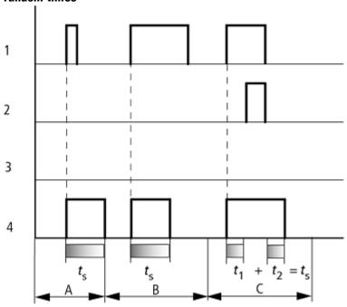
Figure 123: Signal diagram timing relay, single pulse 1
