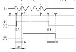
Figure 260: Delay times for evaluating an AC input signal
