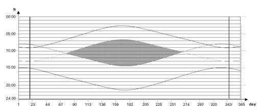
Figure 143: Q1 does not switch on during the winter months
