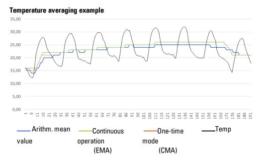
Figure 154: Sample curve for hourly temperature measurement, over 7 days
