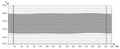
Figure 137: Offset; O1=-2; O2=2; Q1=1 will switch on 2 hours before sunrise and off 2 hours after sunset
