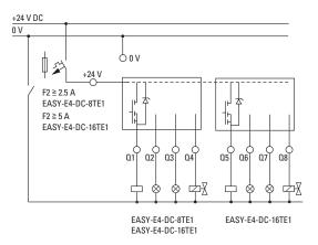
Figure 21: Connecting expansion device transistor outputs
