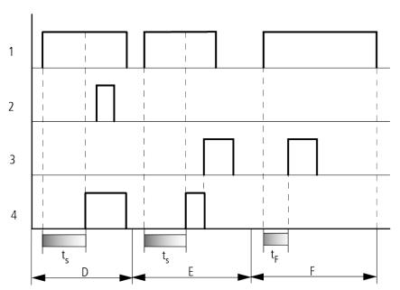
Figure 119: Signal diagram of timing relay, on-delayed (with and without random switching)
