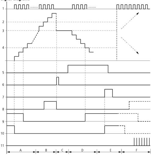
Figure 144: Signal diagram of counter relay
