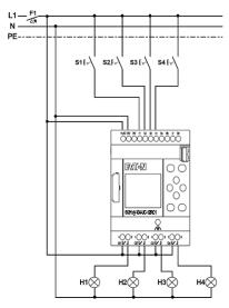
Figure 299: Circuit diagram for easyE4 chaser light
