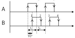
Figure 147: CI function block counting up; QV=QV+4
