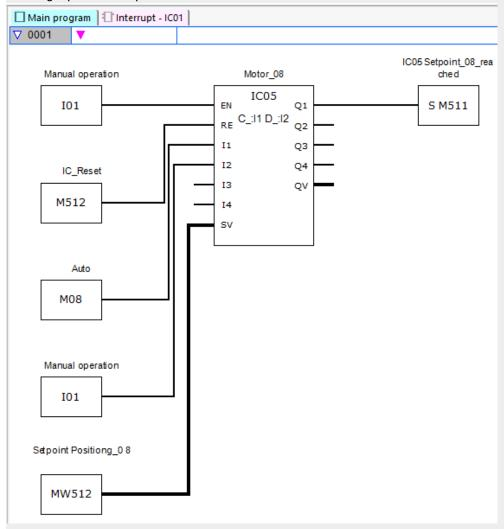
Figure 213: easySoft 7 Main program Incremental counter
