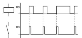
Figure 79: Signal diagram of cycle pulse with rising edge
