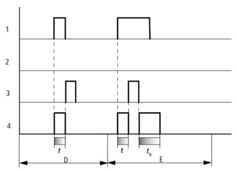
Figure 124: Signal diagram timing relay, single pulse 2
