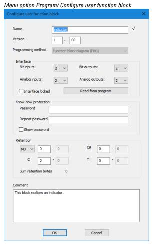
Figure 224: Configure user function block
