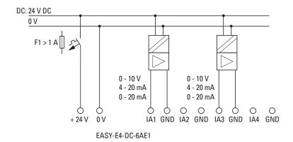
Figure 24: Connecting analog inputs EASY-E4-DC-6AE1
