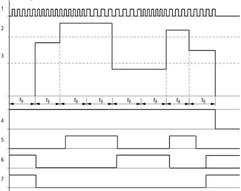
Figure 145: Signal diagram of frequency counter
