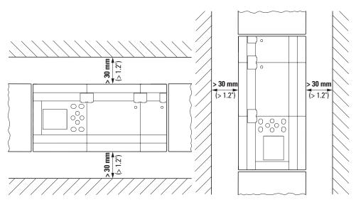
Figure 5: Mounting distance min. 3 cm
