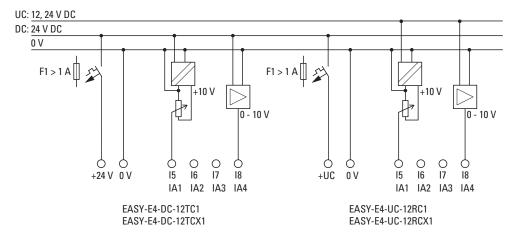
Figure 18: Connecting the analog inputs on base devices
