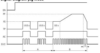
Figure 169: Signal diagram PO pulse output - jog mode
