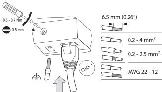
Figure 33: Connecting the Ethernet cable
