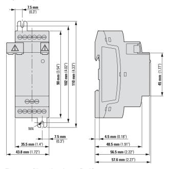
Figure 298: Dimensions in mm (Inch)
