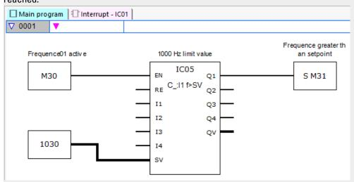
Figure 215: easySoft 7 Main program Frequency measurement
