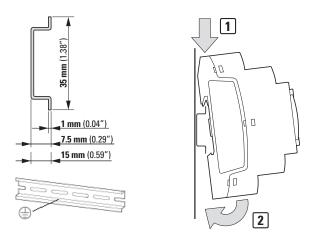
Figure 7: Installation on IEC/EN 60715 mounting rail
