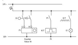
Figure 237: Hardwiring with relays
