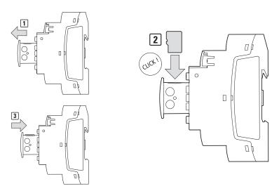
Figure 30: Inserting a memory card
