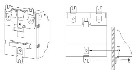
Figure 9: Screw mounting configuration for a device
