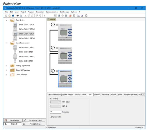
Figure 263: NET configuration without a program
