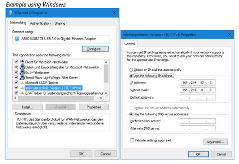
Figure 72: Ethernet connection on PC
