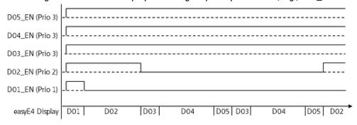
Figure 194: Signal diagram for text display with text function blocks with an identical priority of 3
