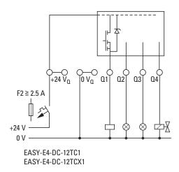
Figure 20: Connecting base device transistor outputs
