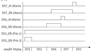
Figure 193: Signal diagram Text display
