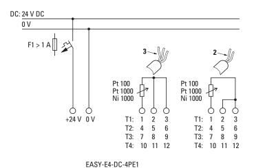
Figure 26: Connecting analog inputs EASY-E4-DC-4PE1
