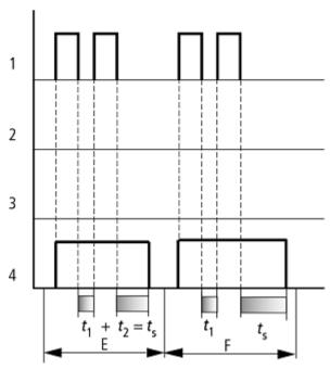
Figure 121: Signal diagram of timing relay, off-delayed
