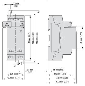
Figure 297: Dimensions in mm (Inch) extensions 2SU
