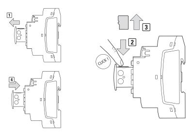
Figure 31: Removing the memory card
