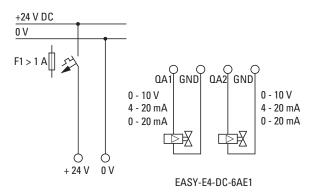
Figure 25: Connecting analog outputs EASY-E4-DC-6AE1
