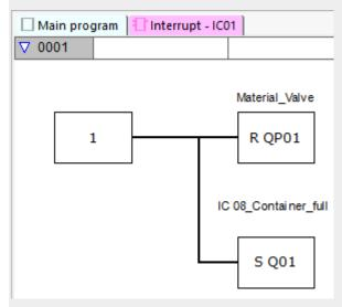
Figure 212: easySoft 7 Interrupt program, two counter inputs
