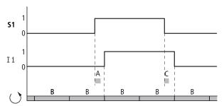
Figure 259: Switching behavior with debounce deactivated
