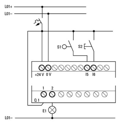
Figure 238: Wiring with EASY-E4-UC-..., for example
