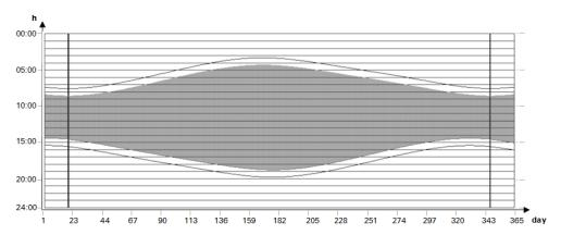
Figure 139: Offset; O1=1; O2= -1; Q1 will switch on 1 hour after sunrise and off 1 hour before sunset
