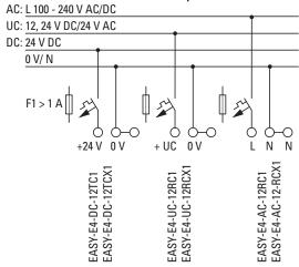
Figure 13: Connecting the power supply for base devices
