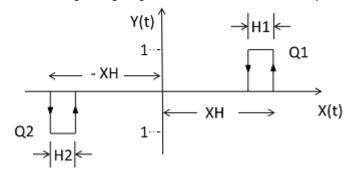
Figure 173: Timing diagram for three-step controller
