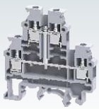
CDL4UN(I.S) 58 x 57.5 x 6 mm 0.2 - 4.0 mm 2 32 A, 800 V, 0.5 Nm
