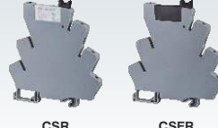
Pitch 6.2 mm CSR Series Coil Voltage: 5 V DC to 230 V AC/DC CSESR Series Input: 24 to 230 VAC/DC Output: 48VDC/4A, 48VDC/100 mA, 380 VAC /2A Standard Screw / Spring clamp
