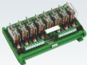
Change Over: 1CO/2CO/4CO No. of Relays: 1/2/4/8/16 Coil volt: DC: 5/12/24, AC: 24A/110A/230A Switching Current: 5 A (2CO/ 4CO) / 10 A (1CO) Max. Switching Voltage: 380 VAC, 125 VDC Standard Screw Terminal (0.5 to 2.5 sq.mm) Standard Din Rail Mounting
