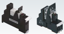
Coil Voltage: DC: 24 AC: 24A/110A/230A Contact: 1CO/ 2CO/4CO Switching Current: 12A (1CO) / 8 A (2 CO) / 5A (4CO) Standard Din Rail Mounting
