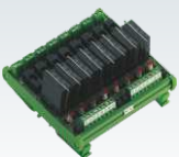
No. of Relays: 1/2/4/8/16 INPUT: 5/12/24 VDC OUTPUT: 2A/100VDC (DC/DC SSR) 3A/400 VAC (DC/AC SSR) Standard Screw Terminal (0.5 to 2.5 sq.mm) Fuse rating up to 6.3 A
