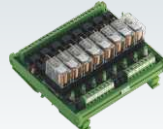
Change Over: 1CO/2CO/4CO No. of Relays: 1/2/4/8/16 Coil Volt: DC: 5/12/24, AC: 24A/110A/230A Switching Current: 5 A (2CO) / 10 A (1CO) Max. Switching Voltage: 380 VAC, 125 VDC Fuse Fail Indication: 24, 110VAC/VDC, 230 VDC/VAC. Standard Screw Terminal (0.5 to 2.5 sq.mm)
