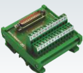
Channels / Pins: 9, 15, 25, 37, 50 Versions: Screw connection, Spring Connection, with LED indication, with component mounting hole. Rated current: 3 A. Standard Din Rail Mounting
