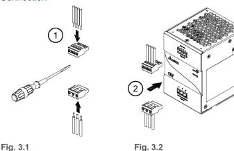
CAUTION: Must tighten wire to housing (Fig. 3.1) before plugging into the terminal block connection (Fig. 3.2).
