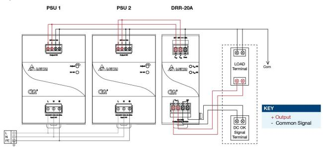
Fig. 4 Redundancy / Parallel Operation Connection Diagram
