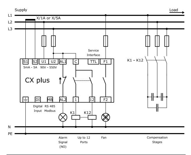
**NOTE:** The CX plus is designed to control **capacitive or inductive** stages. Operating both stage types simultaneously is not possible.
