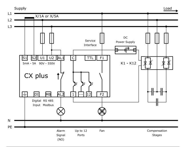
**NOTE:** The CX plus is designed to control **capacitive or inductive** stages. Operating both stage types simultaneously is not possible.
