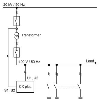
The reactive power caused by the transformer is measured by a medium-voltage current measurement and compensated by the connected compensation system.
