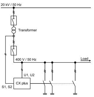
If there are no static stages available to compensate an upstream transformer, this can be done by the control of the CX plus.
