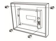
Step 3: Tighten the screws with the torque less than 0.5 N-M / 0.7 N-M to avoid damage to the plastic
