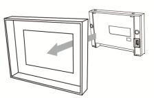
Place the fasteners into the slots and tighten the screws until reaching the panel cutouts.
