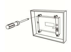
Step 4: For heat dissipation, please keep a minimum clearance of 60 mm on the rear of the HMI.
