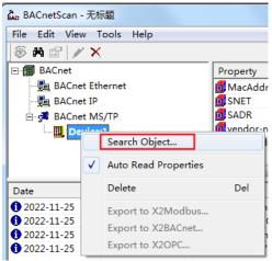
BACnetScan will list all the searched Objects under the Device: 1 option, as shown in the figure below:
