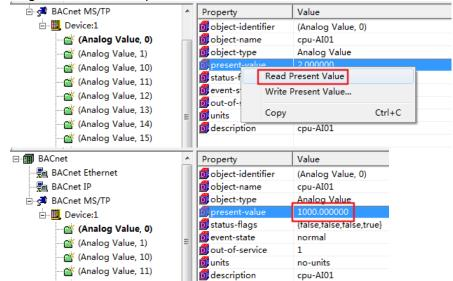
Select the 'Write Present Value' option in the right-click menu to write the value of PLC AF1 as shown in the figure below:
