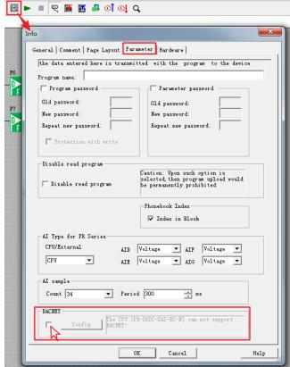
Select the check box, the 'Config' button becomes available, then click this button, the configuration window pops up, as shown in the figure below. Divided into 3 pages: 'Comm', 'Object(BV)' and 'Object(AV)', the following three pages are introduced respectively.
