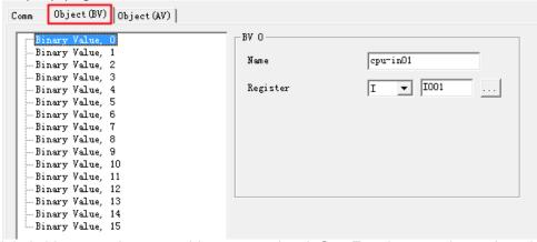
16 digital objects can be set on this page, and an I, Q or F register can be assigned to each object. Registers of type 'I' can only be read, not written. Registers of type 'Q' and 'F' support read/write. But in the program in the PLC, the input pins of their blocks need to be suspended, so that the write operation can be successful.
