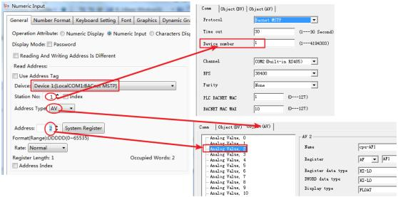
The value of 'Station No.' comes from the 'Device number' in the PLC parameter. 'AV2' is 'Analog Value,2', and so are other registers.
