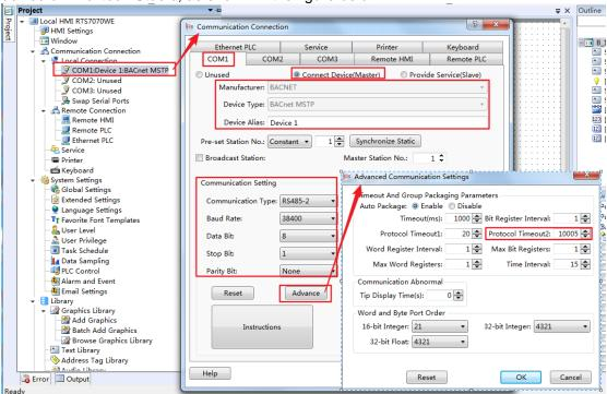
Double-click COM1 under 'Local Connection' and check the 'Connect Device (Master)' option. Select 'BACNET' for 'Manufacturer' and 'BACnet MSTP' for 'Device Type'.
