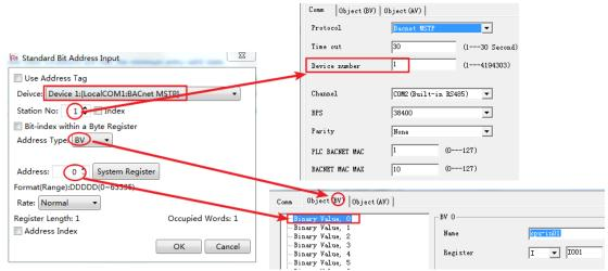
The value of 'Station No.' comes from the 'Device number' in the PLC parameter. 'BV0' is 'Binary Value,0', and so are other registers.
