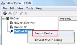
At this time, some prompts will be displayed in the prompt bar, and all found devices will be listed under the option of 'BACnet MS/TP', as shown in the figure below, and the message bar will prompt 'BACnet MS/TP 'Device: 1' is found'.
