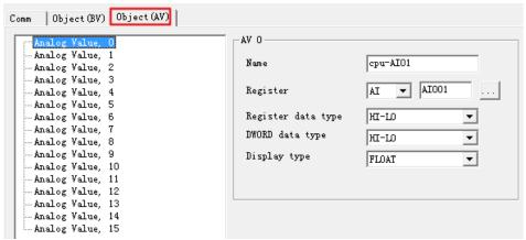
Similarly, 16 analog objects can be set on this page, and an AI, AQ, AF or VW register can be assigned to each object. The 'AI' register can only read values, but cannot write values. AQ, AF and VW support read/write, and only when the input pins of these register blocks are floating, the write value operation can be successful.
