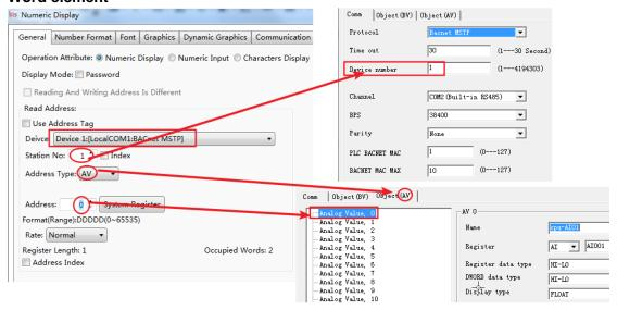
The value of 'Station No.' comes from the 'Device number' in the PLC parameter. 'AV0' is 'Analog Value,0', and so are other registers.
